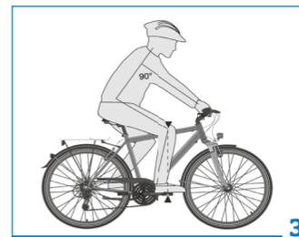
When one pedal is forward, the knee is over the axle of the front pedal (see "Illustr.: Optimum seating position (3)").
