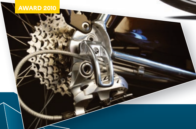
Q-guard quick release with integrated derailleur protector. Integrating the two functions results in a new innovative component both lighter and more attractive than the two separate items.
